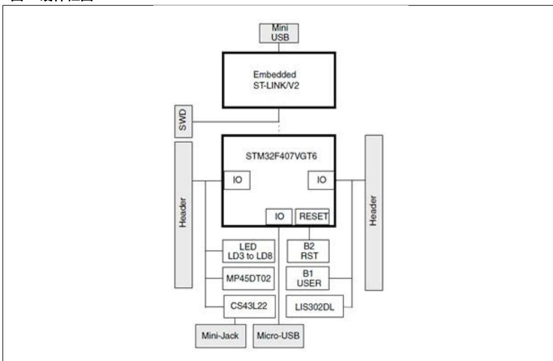
**图 3 顶层布局**
